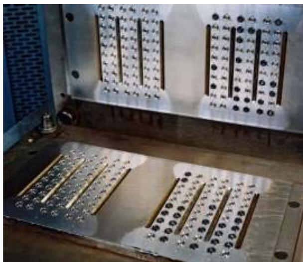
Figure 2. O-ring mold used for demolding tests
